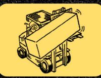
Take special care when carrying a long or wide load. Turn and work slowly to prevent the load from shifting. Make sure the load is balanced.
