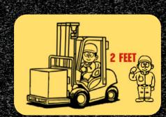
An operator who stops a forklift or other mobile equipment to speak to a pedestrian must abide by the "2-Foot Rule." This rule requires an operator to maintain a minimum distance of 2 feet (or outstretched arm's length) between the forklift or other mobile equipment and the pedestrian being spoken with.
