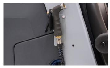
Apply solution to the floor in conjunction with vac wand, or used for machine cleaning. (optional)
