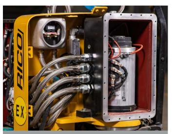
**FLEXIBLE CONDUIT (FC) CABLES** house regular cabling, which is sealed to ensure safe use in an EX-rated environment. The FC Cable provides flexibility and space saving.
