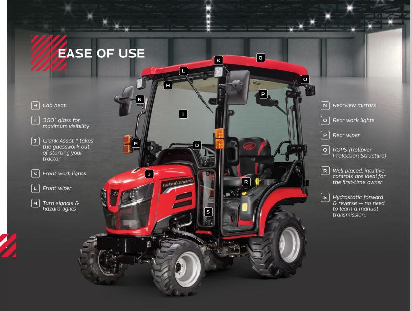
The Mahindra 1100 Series ROPS cab (Rollover Protection Structure) is designed, fabricated, and fitted at our assembly plant. It can be heated quickly and efficiently to provide warmth on extremely cold days. Additionally, the glass-enclosed cab provides a 360-degree view and includes work lights, mirrors, and wipers to deliver an exceptional experience, setting a new class standard.
