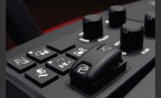
On cab models, the electronic rear hitch controls improve chore efficiency and overall productivity. Easily adjust lift speed, draft, depth, auto-raise on turns, & more.
