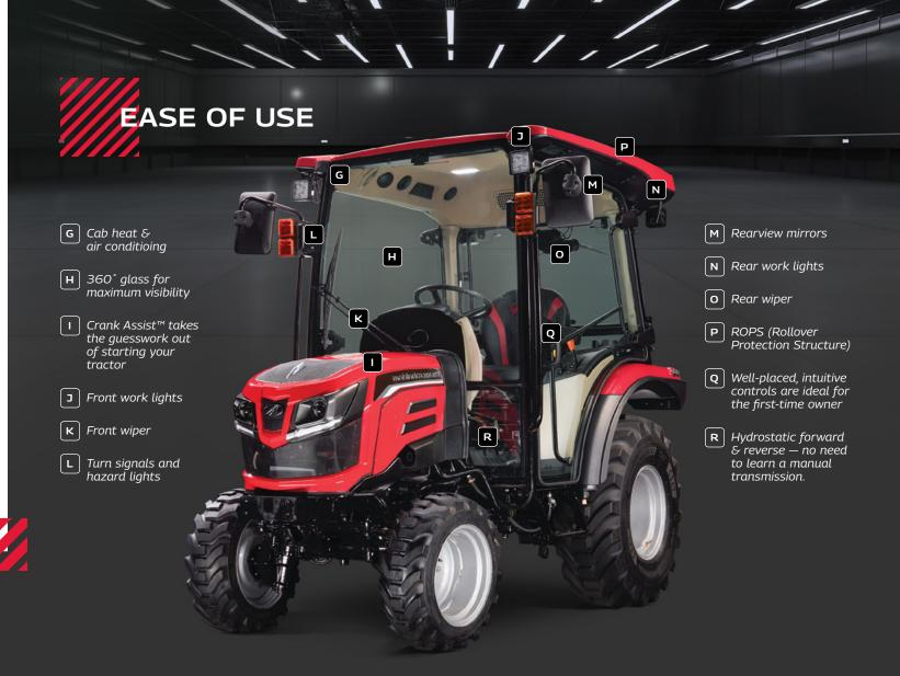
The Mahindra 2100 Series ROPS cab (Rollover Protection Structure) is designed, fabricated, and fitted at our assembly plant. It offers a comfortable ride all year round with built-in heat and air conditioning. Additionally, the glass-enclosed cab provides a 360-degree view and includes work lights, mirrors, and wipers to deliver an exceptional experience, setting a new class standard.
