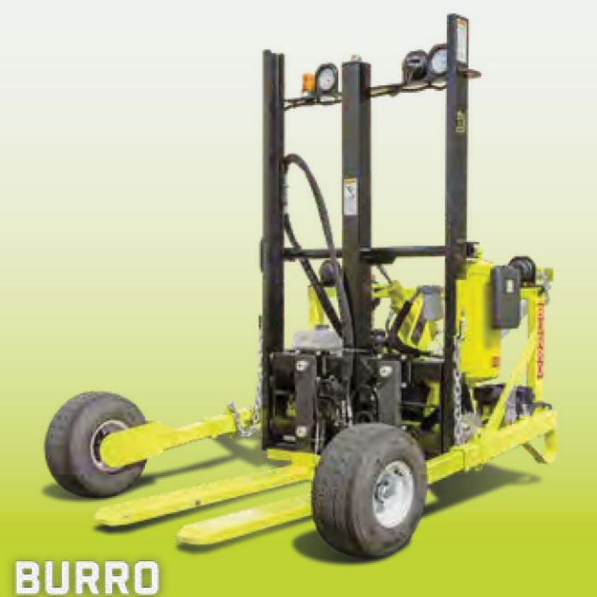
Better than an all-terrain pallet jack, our Burro Truck Carried Forklift is your best solution for smaller jobs. At only 1,800 lbs, the Burro lifts 3,000 lbs to 65 inches.
